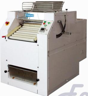
The equipment processes your batch of dough automatically without the intervention of the operators. The roller gap & processing time can be predetermined by the operators. When the process is done, the timer will activate the discharge chute to be open and the dough sheet will be discharge out.
