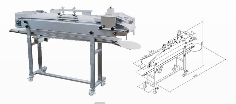
Put the well divided dough into the hopper, The bagel will be formed automatically.
