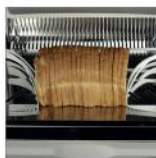
JAC FLAPS Holds the loaf together for easier handling at the exit of the slicer.
