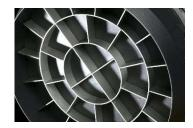
Anodized coated aluminium dividing disc and stainless steel knife require minimal flour for dividing and are hygienic in use.
